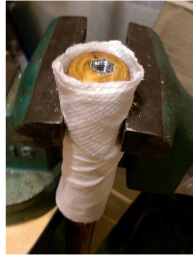
Figure 3: Stick wrapped in paper towel and clamped in a vise.
