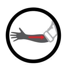
Always wear short sleeves, or rolled sleeves, pull back and tuck in long hair, remove jewelry and lanyards, etc. Do not wear gloves.
