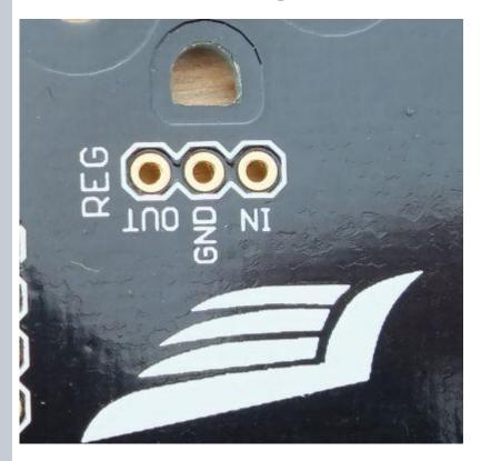
If you need a external regulator for your camera o for your video transmitter, then solder your video regulator there. It should match with the pololu regulators. Any other regulator could be solderd there, but maybe it doesn't fit as well. For common setup you dont need this.
