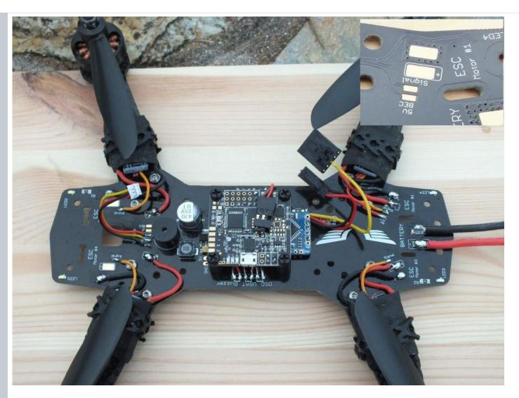
Last but not least, connect your ESC to the pdb. Just place the red wire into the (+) pad, and the other its ground connected to your black wire.
