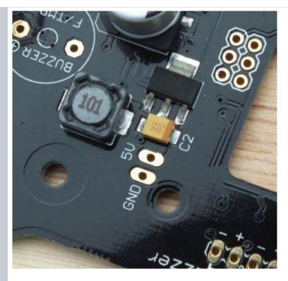
You have a 5v pads on the PDB to connect other things on it. For example leds strips. Connect the VCC of you led strip there in the 5V, and the GND on the GND pad. The signal or DIN into your flight controller pin 5 (using PPM SUM). But remember that you can handle only 1A on the onboard regulator, so if you have plans to place a lot of leds, or power severals things on it, maybe its better to use the BEC of other ESC to make this.
