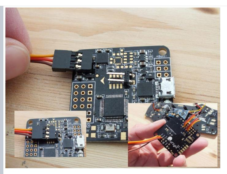
Depeding on your flight controller, you have to solder pin headers to it or not. But to make a good clean setup, i usually solder the wires directly on the flight controller. Other clean metohd could be use angled pin headers, but not any flight controller support this.
