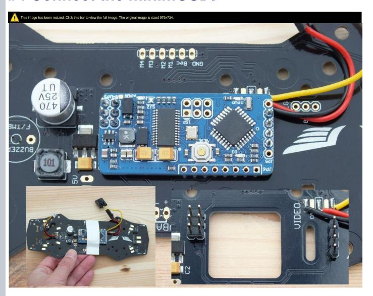
Start to solder the vertical pin headers in place. Then attach the OSD before solder anything, and place the OSD with tape. With this metohd your pins will match perfectly to your osd, and they wont move during solder.
