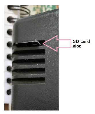
The unit is controlled by the configuration stored on an SD card inserted at the side of the unit. This needs to be in the unit at all times for full functionality.
