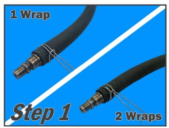
Cut a length of wire that is about four times the circumference of the hose plus 1 foot (~30cm).
