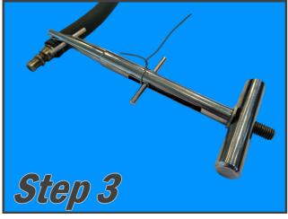
Now twist the tension handle to tighten the wire. You will feel the wire pull tight and stop twisting once it goes firm.
