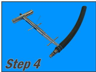
Now you just need to flip the Wire Clamp over to bend the wires over the loop.
