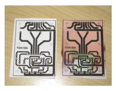
Step 4: Ironing The Printed PCB Layout
