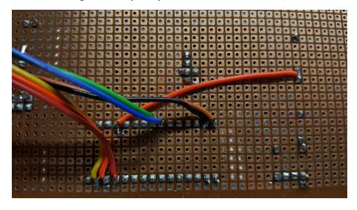
5.1.6:Connect the power wires from the Buck converter (+ , -) to Arduino Nano (VCC , GND).
