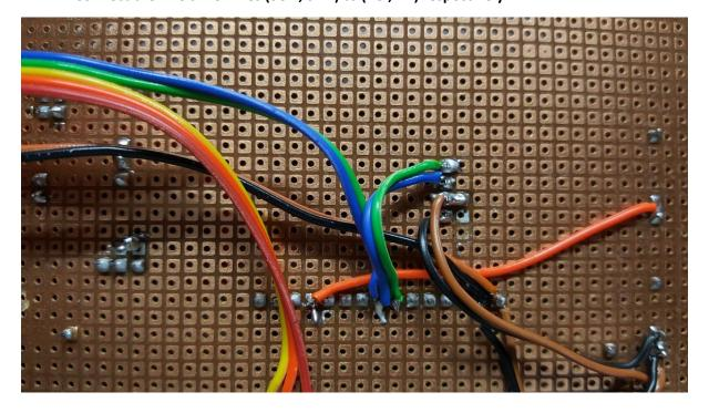
Connect one of the Relay terminals to the transistor's Collector
