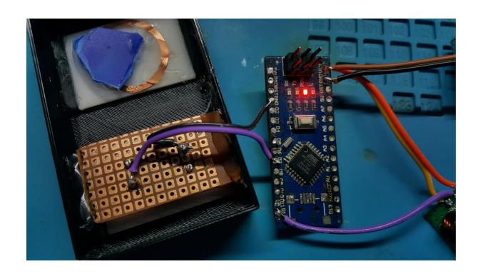
4.1.15: Prepare the antenna : Cut 17.3cm of wire
