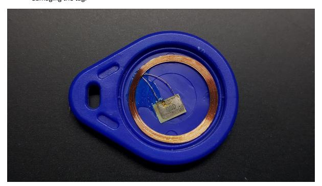
After opening it, I trimmed all of the plastic (blue), leaving the parts where it is glued.
