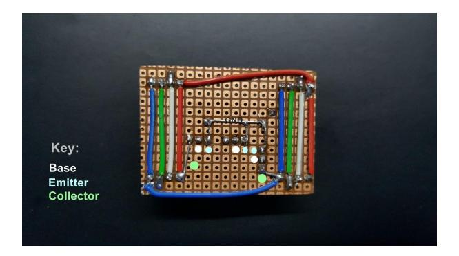
Once it is done, Connect the collector terminal of the Green LEDs' transistor (the middle one) with a silvered copper wire that connects the transistor's collector to the Green LEDs' Terminal. (Like shown in the images)
