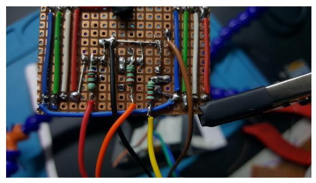
\*You may add heat shrink tube to the resistor terminals, but I hadn't as its going to be enclosed in an enclosure anyway.
