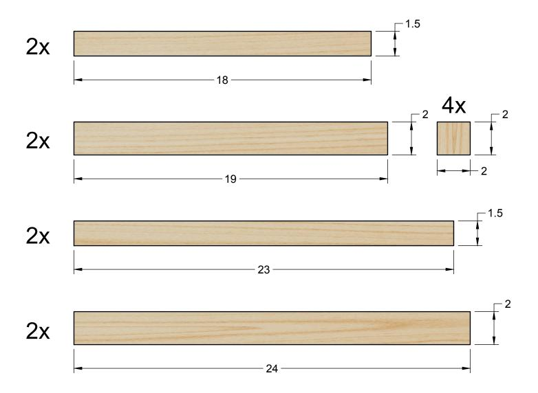
Adjustable Juice Groove Jig Parts from <sup>1</sup>/<sub>2</sub>" Plywood
