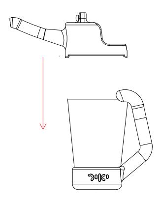
Insert body number 2 into the upper part of the cup, lock the upper part with the handle of body 1
