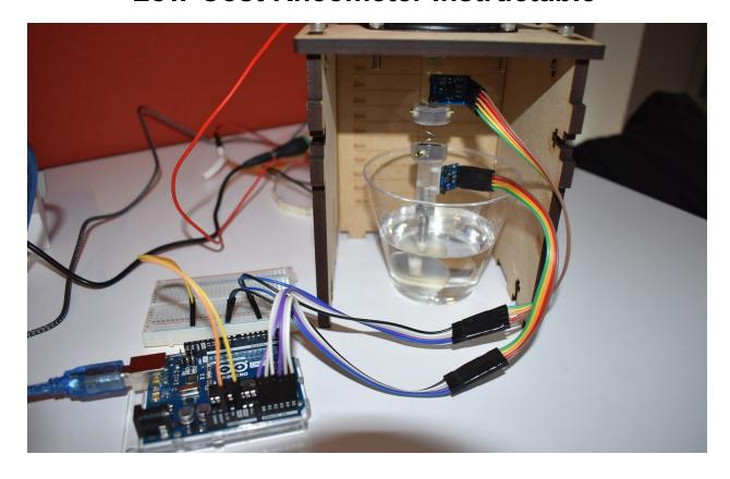
The purpose of this instructable is to create a low cost rheometer to experimentally find the viscosity of a fluid. This project was created by a team of Brown University undergrad and graduate students in the class Vibration of Mechanical Systems.
