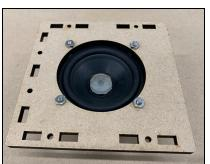
Final step of the set-up -- putting it all together! Start by unclipping the alligator clips from the speaker and screwing the speaker into the top of the housing assembly with the 6-32 x  $\frac{1}{2}$ " Hex head screws,6-32 hex nut and the 9/64" Allen Key. Next, screw the vibrating mass assembly (with the accelerometers) into the speaker. For the best result, we recommend turning the speaker to avoid tangling the accelerometer wires. Tighten the mass to the speaker with the aluminum hex nut.
