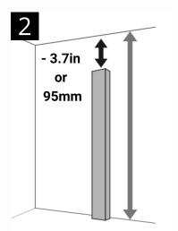
Measure the ceiling height and minus 3.7 inches or 95 mm from the ceiling height.
