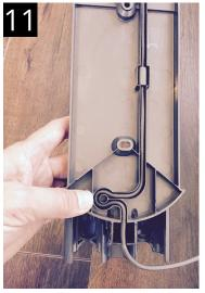
Attach the charging cable to the docking station.
