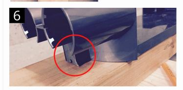
Align the docking station over the pilot holes.
