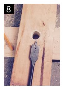
Use a ¾" paddle/spade drill bit to bore a hole through the timber.
