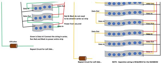
NOTE: Sepentine wiring is REQUIRED for the RAINBOW LEDs Set. This must be done to match the programming. VU Meter also must be wired this way.
