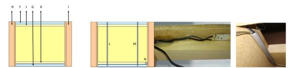
Cut two round steel rods L and M of 5 mm. diameter to a length of 340-8 = 332 mm. and place them in the holes of the front and back as shown on the drawing. Glue to the bottom of part K the 27 cm. LED strip and secure the wiring with glue. Glue the aluminum tube N in the right inner corner for the wiring of the LED strip under part K and the LED strip that will be mounted inside the picture frame.
