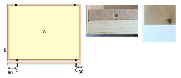
The sand holder consists of a base plate (A) with a slat (B) of 9x9 mm. glued to the edge. The corners of this slat are cut at 45 degrees to ensure a good fit. At the bottom of the long sides are 2 mm. metal pins mounted to fix the holder to the housing.
