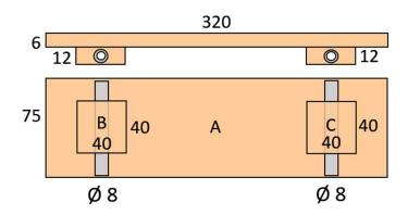
The base plate A has the same dimensions (length and width) as the base plate of the X-carriage. Carefully drill an 8 mm. hole with a drill press perpendicularly through the center of the side of both guide blocks B and C. First do this with a small drill and finally with an 8 mm. drill, otherwise the MDF material may crack. Mount an aluminum tube in each block. Then mount both blocks under the base plate A is as follows:
