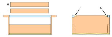
Finally, glue the MDF strips J and K on the inside at the top to the pinewood slats according to the drawing.
