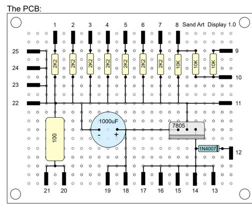
Mount the Arduino in the control panel with three M3 bolts, using two nuts per bolt as spacers. Build the parts print on the PCB according to drawing with all shown parts. Solder the connections for the wiring at the top side of the PCB so the wiring can be connected easy. Mount it next to the Arduino on the bottom plate of the control panel with four wood screws using M3 nuts as spacers.
