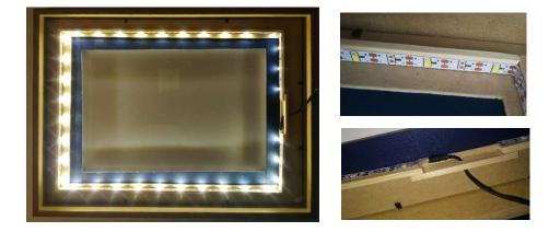
Glue the LED strip on the inside of the 9x4 mm. slat, solder 50 cm. flexible wiring to the strip, glue this on the wood with a shrink sleeve protection to prevent damage. The led strip is just a few LEDs too short, so solder a part of a second strip to it. Of the remaining LEDs, a few are glued in the housing at the top under the part K so that the mechanism of the display is also illuminated. The LED strip can easily be cut on the oval copper surfaces and soldered together.
