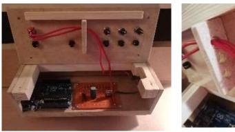
Glue a pinewood slat 9x9 mm. to the bottom of the lid with a length of 150 mm. to lock the lid so it fits snugly. Glue a small MDF board with three 8 mm. holes, dimensions 40x15 mm. and 6 mm. thickness at the bottom of the lid. This is used to guide the wiring.
